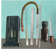
Fig. 6.3: Sahlb's hemoglobinometer showing the box with standard color, diluting tube, pipette, glass rod, N/10 HCl and dropper
