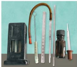
Fig. 6.1: Sahl's hemoglobinometer showing the box with standard color, brush, diluting tube, pipette, glass rod, N/10 HCl and dropper.
