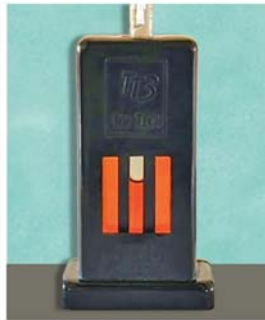
Fig. 6.3: Correct matching of sample with standard color.
